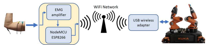
Figure 3 Overall system architecture
