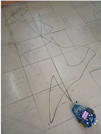
Fig. 3. Cell visit indication with a black line.
