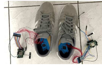
Fig. 4. Smart Insole system inside a pair of shoes
