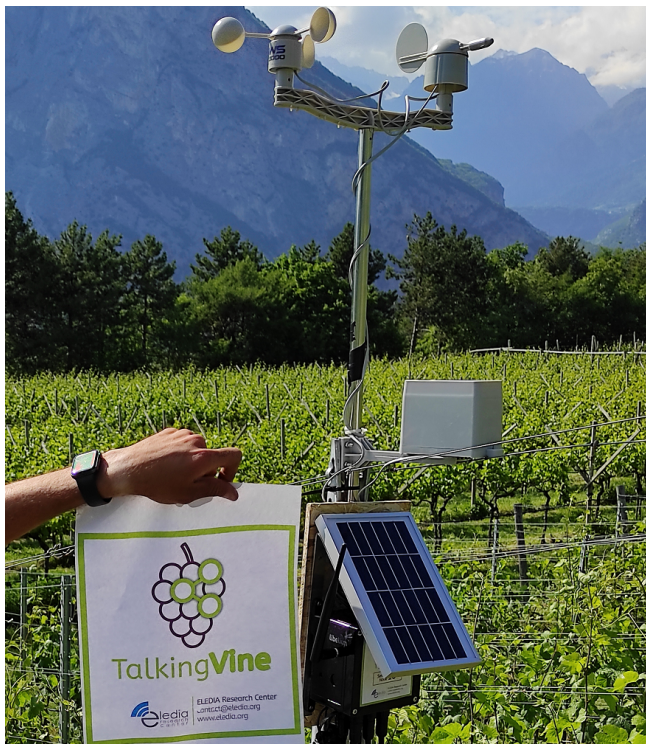
Fig. 2. A wireless sensor node installed in the experimental validation site. The sensor is also equipped with a weather station and a solar panel.
