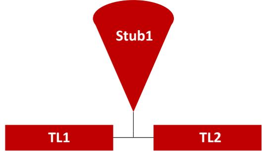
Fig. 3: Impedance matching network. TL1, TL2 and Stub1 are the rectangular and radial stubs accordingly
