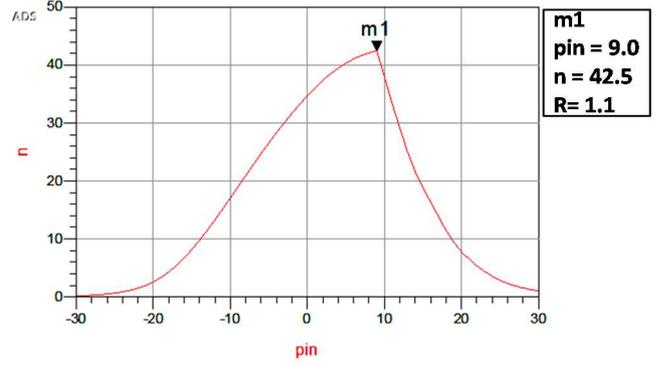
Fig. 7: Power conversion efficiency (%) - Pin (dBm) at 3.5 GHz for  $R_L = 1.1K\Omega$
