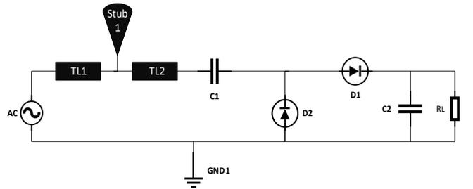
Fig. 4: Total design of proposed rectifier
