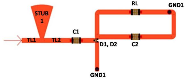
Fig. 8: Layout of the rectifier
