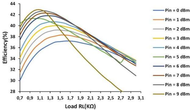
Fig. 6: Power conversion efficiency (%) - output load RL (K $\Omega$ ) at 3.5 GHz for various Pin values
