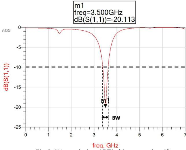
Fig. 5: S11 magnitude and BW of the proposed rectifier
