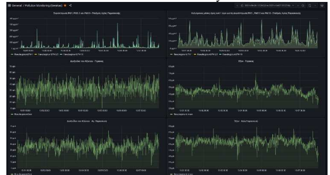
Figure 7. Grafana, concentration of PM2.5, Nitrogen dioxide (NO 2 ), Ozone (O 3 ) from two low-cost stations.
