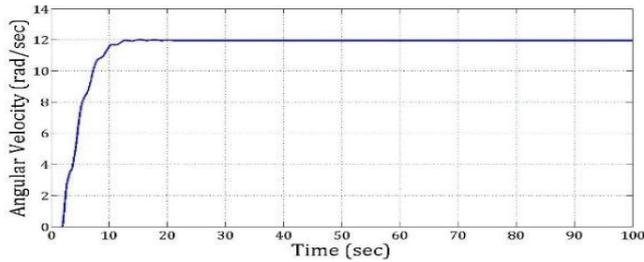
Fig. 6. System response for settling time<10 sec and overshoot<5%
