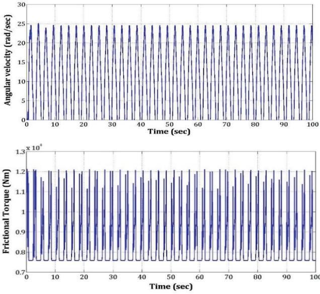
Fig. 1. Simulation of torsional vibrations for  $\Omega_0 = 12.5$  rad / sec (angular speed of drill bit and friction torque)
