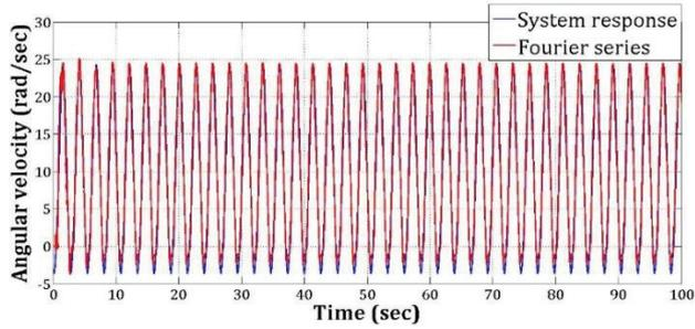
Fig. 2. System response and Fourier approximation for the angular velocity of the bit
