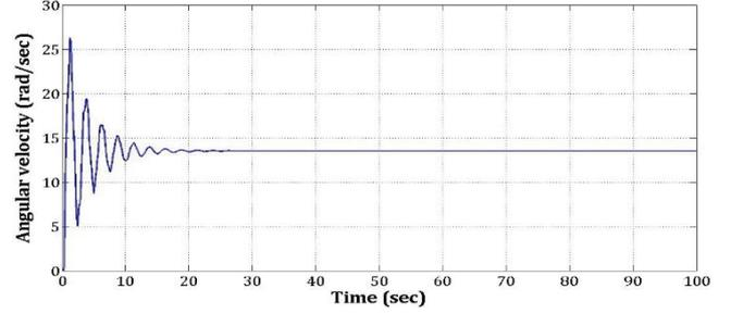
Fig. 4. Simulation of torsional vibrations for WoB=40kN
