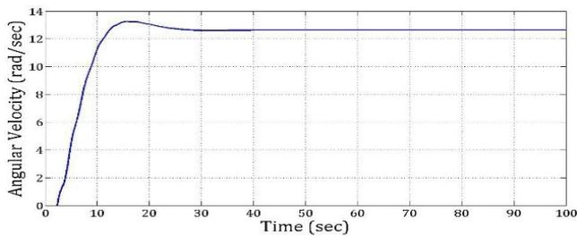
Fig. 7. System response for settling time<20 sec and overshoot<10%
