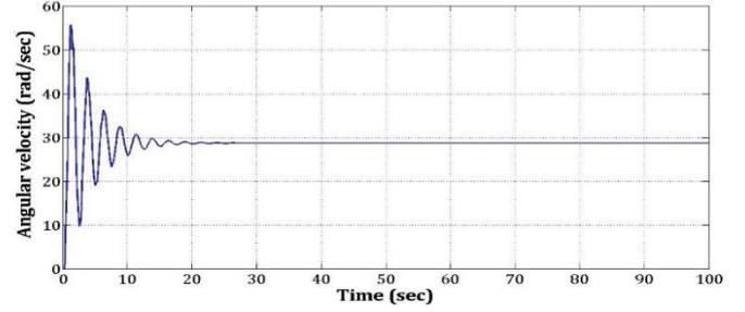
Fig. 5. Simulation of torsional vibrations for  $\Omega_0=30$  rad / sec
