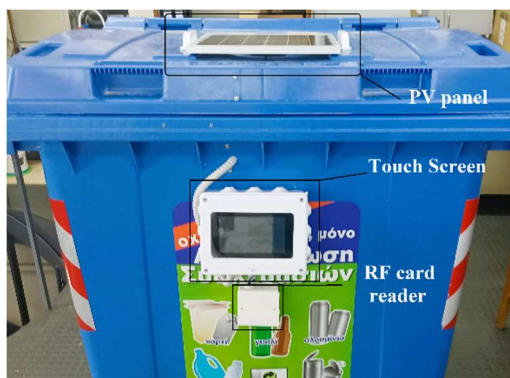
Fig. 8. Front view of the installed smart kit, at a conventional recycling bin.
